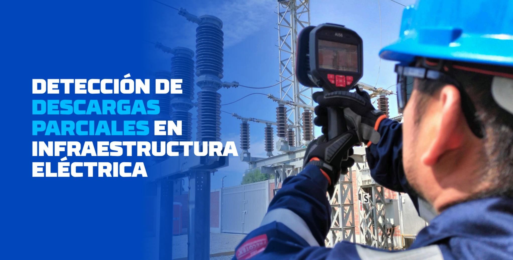
A close-up, over-the-shoulder view of a worker in a blue hard hat and safety glasses using a handheld ultrasonic detector. The worker is wearing a dark blue jacket with a red and white logo on the sleeve. The detector has a screen and several red buttons. The background shows an electrical substation with large insulators and metal structures under a clear blue sky.
